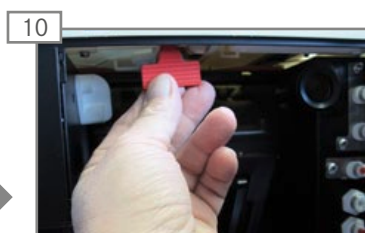
Push the locking slide all the way to the rear.
